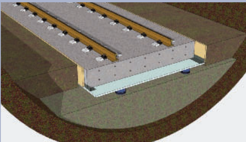
Picture 5: MSS in tunnel
